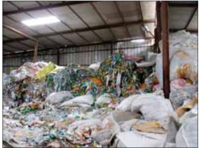
Multilayer plastics waste waiting to be converted into Chipboard (Deluxe Recycling (India) Pvt. Ltd.).
