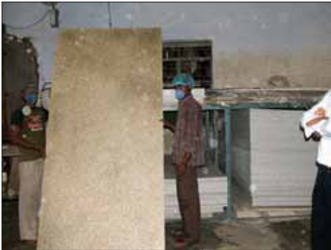
Chipboard made out of multilayer plastics waste (Deluxe Recycling (India) Pvt. Ltd.).
