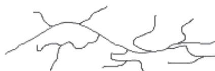
A molecule of branched polyethylene, or LDPE
