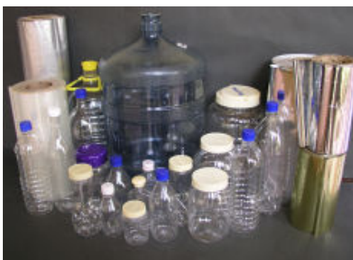
Fig. 2. 3. PET based food packaging materials (films/laminates/containers)
