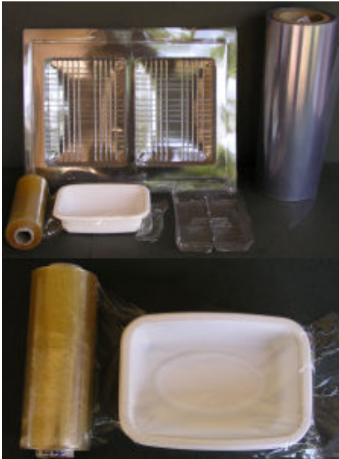
Fig. 2.2. PVC based food packaging materials (Thermoformed/Clingwrap)
