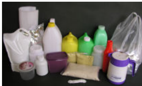
Fig. 2.1. Polyolefin based food packaging materials
