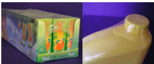
Fig. 4.7. Shrink wrapping of aseptic fruit juice packages and HDPE container.
