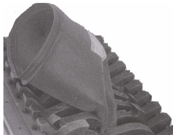
Figure2: Size reduction of a PE drum in an industrial shredder.
