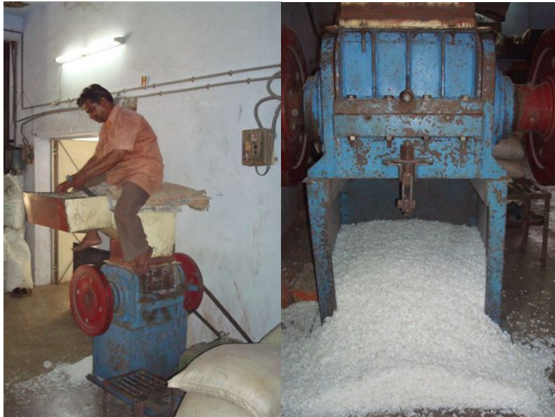
Manual feeding where no safety maintained
