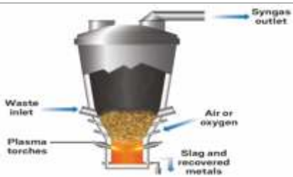
Figure 27- Gasification Plant (Source Chemical & Engineering News)
