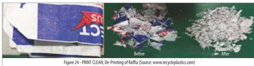
Figure 24 - PRINT CLEAN; De-Printing of Raffia (Source: www.recycleplastics.com)
