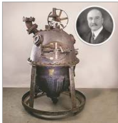
Picture 3- Bakelizer, used by Baekeland (1907- 10) to form Bakelite. Source https://www.sciencehistory.org/historical-profile/leo-hendrik-baekeland
