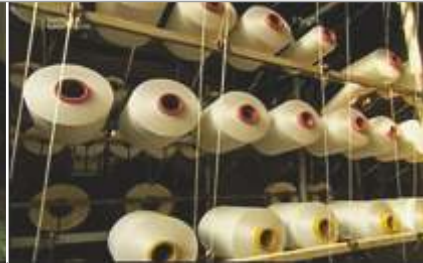
Figure 19- Polyester Fiber being wound on Bobbins (Source: National Geographic)
