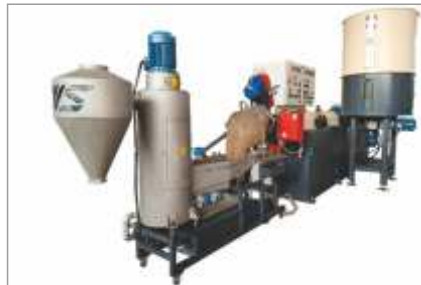
SSFigure 17- Schematic of Single Screw Forced Feeder Type Recycling Extruder (Source https://www.recycleplastics.in )
