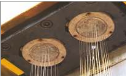
Figure 20 -Extrusion through a spinneret (Source - You Tube)
